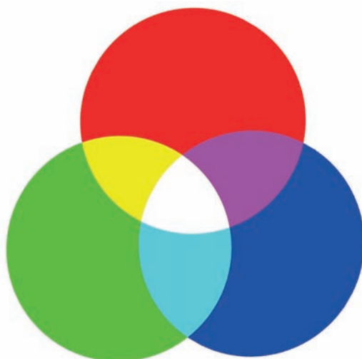
Figure 8.3. Color wheel showing how cyan, magenta, and yellow are obtained by combining red, green, and blue.
